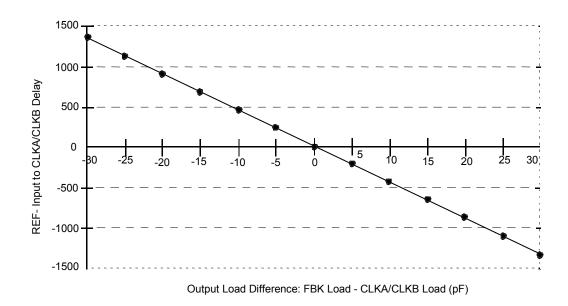
To close the feedback loop of the ASM5P2308A, the FBK pin can be driven from any of the eight available output pins. The output driving the FBK pin will be driving a total load of 7 pF plus any additional load that it drives. The relative loading of this output (with respect to the remaining outputs) can adjust the input output delay. This is shown in the above graph.
