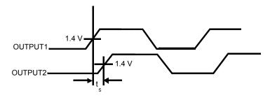
**Input - Output Propagation Delay**
