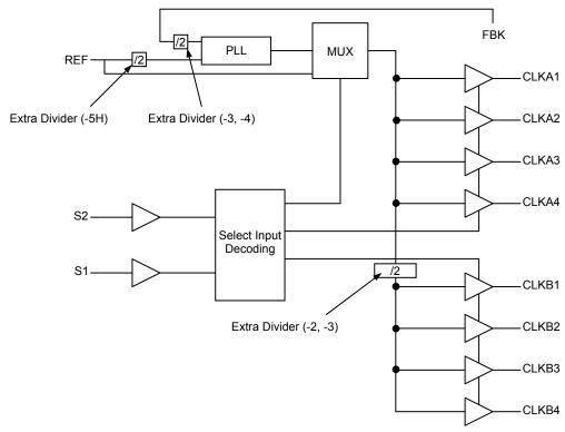
Select Input Decoding for ASM5P2308A
